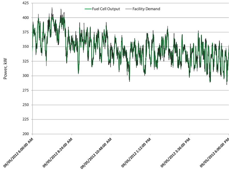
Figure 3. Load-Following Operating Data for Net Metering Site
